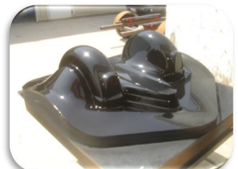
This high-gloss coated, polished, buffed plug is ready for mold manufacturing. Photo Credits: RTM North
