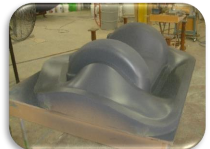
After hand-working the plug surface, an easy-to-smooth coating is applied and sanded to size and surface.
